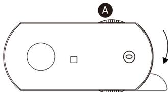
Rotate selector knob **A** to the position of desired circuit.
