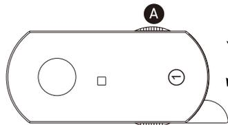
**Circuit 1:** Rotate the knob **A** 90° clockwise from the starting position OFF, to connect circuit 1.
