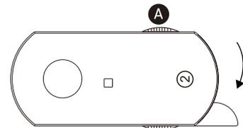
**Circuit 2:** Rotate the knob **A** 90° anti-clockwise from the starting position OFF, to connect circuit 2.
