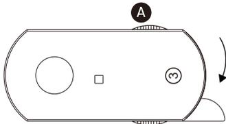
**Circuit 3:** Rotate the knob **A** 180° clockwise from the starting position OFF, to connect circuit 3
