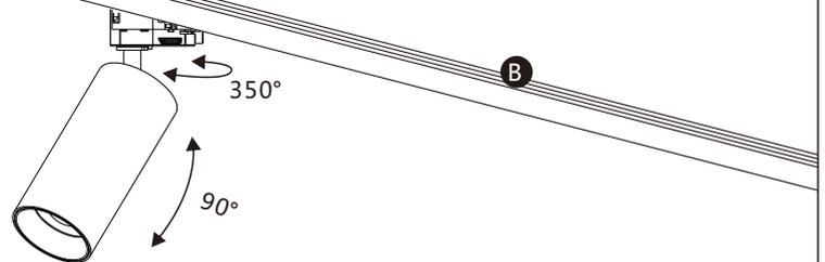
The installation is complete, support can be freely rotated 0°-350° the lamp body can be freely rotated 0°-90°.
