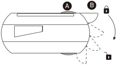
To mount the track adaptor into the track system, first check that the selector knob **A** is at OFF position and the adaptor lock **B** is disengaged.
