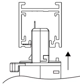
When installing the adaptor into the track, ensure that it is orientated correctly.
