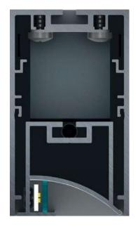
The asymmetrical light effect can evenly cover an entire wall from a distance of as small as  $^{1}/_{5}$  of the height of the wall, assuring visual comfort while avoiding glare and shadow projection on the wall.
